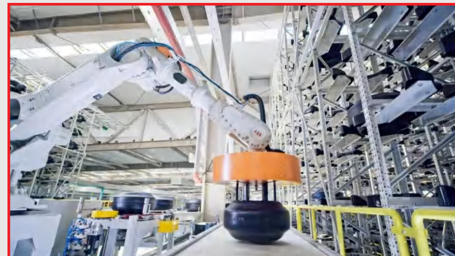
Green tire automatic logistics transportation system
